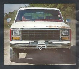
Ford F150 4x4 pickup makes use of Ramsey custom bumper mounting kit. shown here with optional chrome bumper. Ramsey mounting kits require no frame cutting or welding and bott easily in place on your vehicle.
