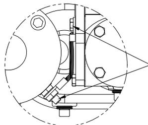
JUMPER CABLE (#440315) MUST BE INSTALLED ON WINCH FROM MOTOR ISOLATED GROUND STUD TO GEAR HOUSING COVER BOLT AS SHOWN FOR NON GROUNDED CHASSIS APPLICATIONS.
